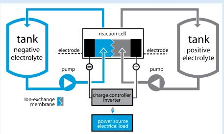
A vanadium redox flow battery is a type of rechargeable battery in which the energy is stored chemically in liquid electrolytes. Unlike conventional batteries, that store all of their reactive materials within the cells, a flow battery stores the electrolytes in tanks. The electrolytes are pumped through the cells and back into the tanks when the battery is active.
